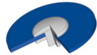
Diaphragm made of rubberized fabric
